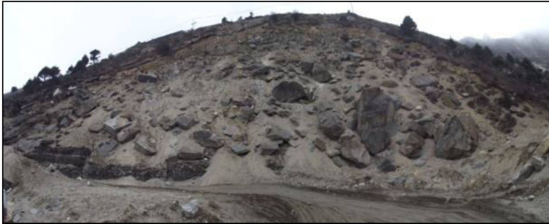
Picture 7 Loose to variably compacted boulder laden Debris- the dominant Surficial Material
